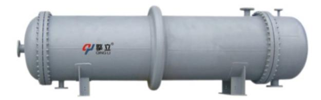
Shell and tube heat exchanger combined with Flange, connecting flange of cooling water, shell, tubular, shell cover, connecting flange of supplies inlet and outlet. There are many types of the heat exchanger tube material such as carbon steel tube, stainless steel tube, titanium tube, copper tube,ripple titanium tube etc.
